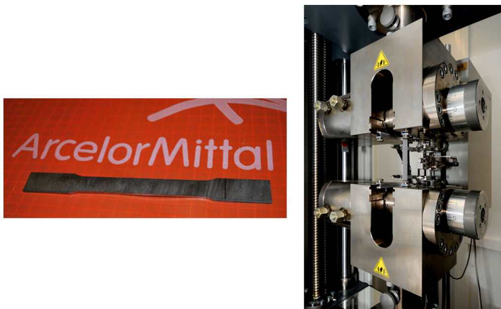
Figure 13: ISO 20/80 specimens and detail of the tensile test machine
