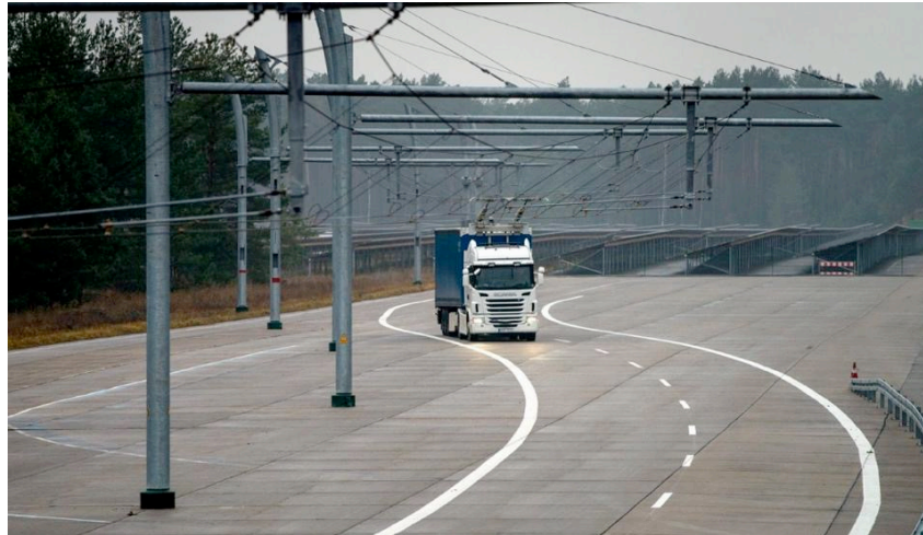
Figure 3. eHighway for freight transport developed by Siemens
