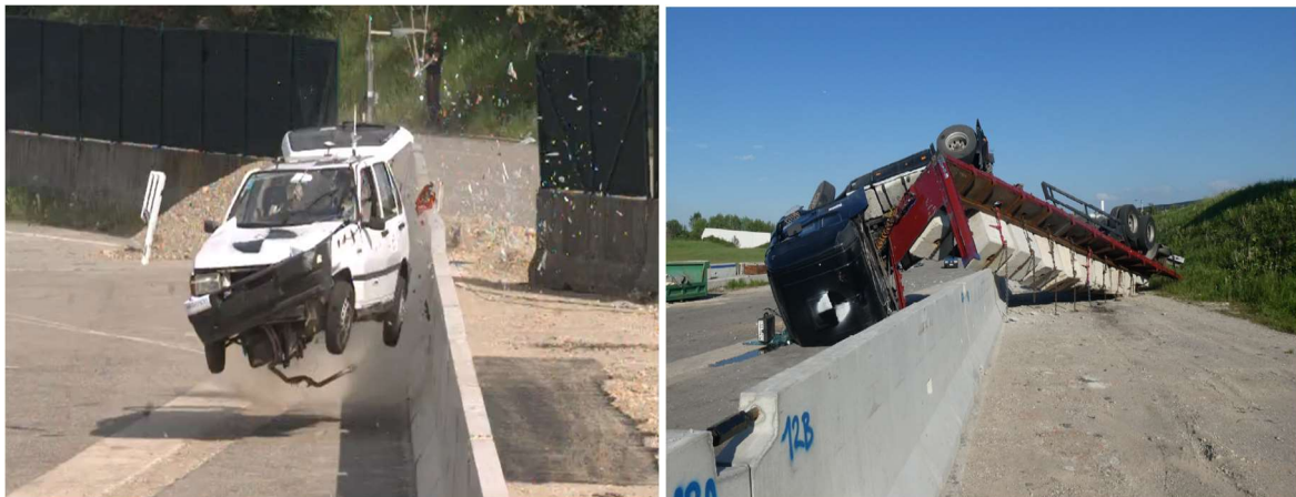
Figure 3 - TB11 crash test result ASI value 1.53 (left), TB81 crash test result with rolled over crash vehicle (right)
